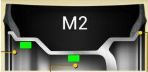
Model two: icon(M2), the system is under the balance model of M2, and the choose of the compensating side is shown as the icon, and we can stick the unbalance block on the two compensating sides by the inner side of the rim's spoke.
