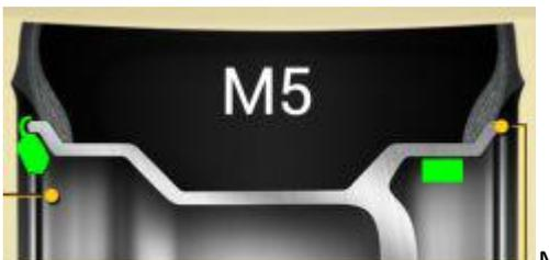
Model five: icon(M5), the system is under the balance model of M5, and the choose of the compensating side is shown as the icon, and we can clamp the unbalance block at the side of the compensating side by the inner side of the rim, and stick it to the compensating side by the outer side of the spoke.
