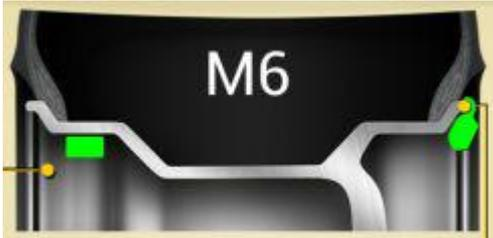
Model six: icon(M6), the system is under the balance model of M6, and the choose of the compensating side is shown as the icon, and we can stick the unbalance block to the compensating side by the inner side of the rim's spoke, clamp it at the outer side of the spoke.
