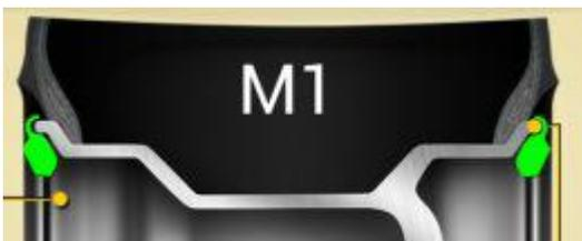
Model one: icon(M1), when it has a yellow frame, it means the system is under the balance model of M1, and the choose of the compensating side is shown as the icon, and we can clamp the unbalance block at the compensating side on two sides of the rim.
