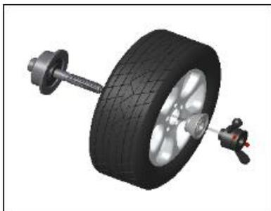
Main shaft - Wheel (installing face of rim forward inside)-
