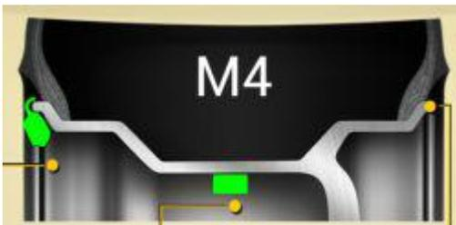
Model four: icon(M4), the system is under the balance model of M4, and the choose of the compensating side is shown as the icon, and we can clamp the unbalance block at the side of the compensating side by the inner side of the rim, stick the unbalance block on the compensating side by the outer side of the rim.
