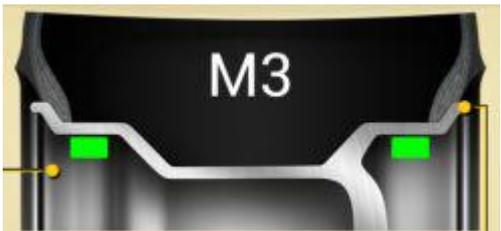
Model three: icon(M3), the system is under the balance model of M3, and the choose of the compensating side is shown as the icon, and we can stick the unbalance block on the two compensating sides by both inner and outer side of the rim's spoke.
